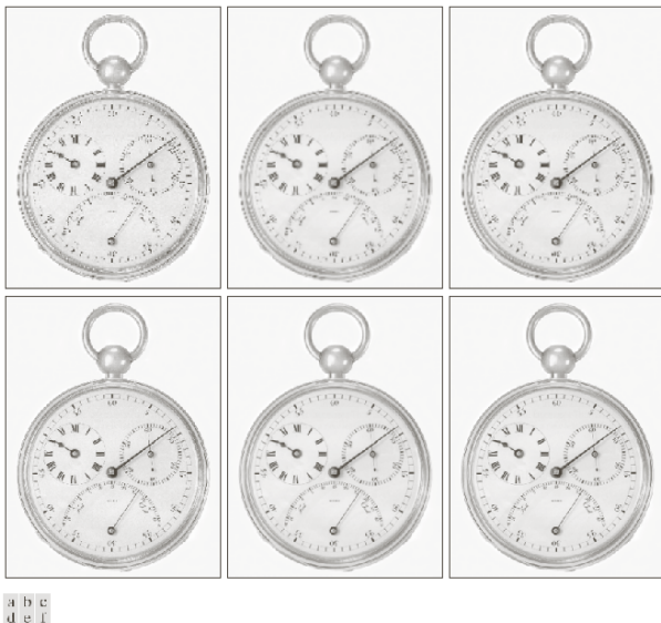
FIGURE 2.24 (a) Image reduced to 72 dpi and zoomed back to its original size ( 3692 \times 2812 pixels) using nearest neighbor interpolation. This figure is the same as Fig. 2.20(d). (b) Image shrunk and zoomed using bilinear interpolation. (c) Same as (b) but using bicubic interpolation. (d)–(f) Same sequence, but shrinking down to 150 dpi instead of 72 dpi [Fig. 2.24(d) is the same as Fig. 2.20(c)]. Compare Figs. 2.24(e) and (f), especially the latter, with the original image in Fig. 2.20(a).
