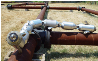
Explorer can traverse pipe networks and 6-to-8 inch pipes
